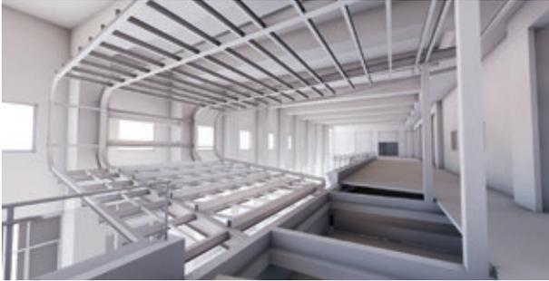
The proposed architectural shape and geometry of the theatre overhangs from the existing concrete balcony level, cantilevering by approximately eight meters and providing an illusion that the theatre is floating.
