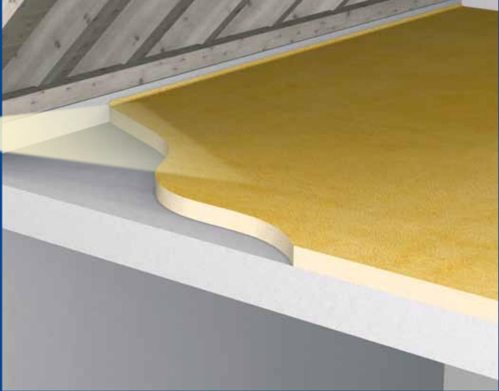
Thermal insulation of the ceiling of a concrete framed building is the most simple and cost effective solution in energy conservation, if the top floors of the building are occupied. This is assuming the roof void remains unheated or not converted into living quarters.
