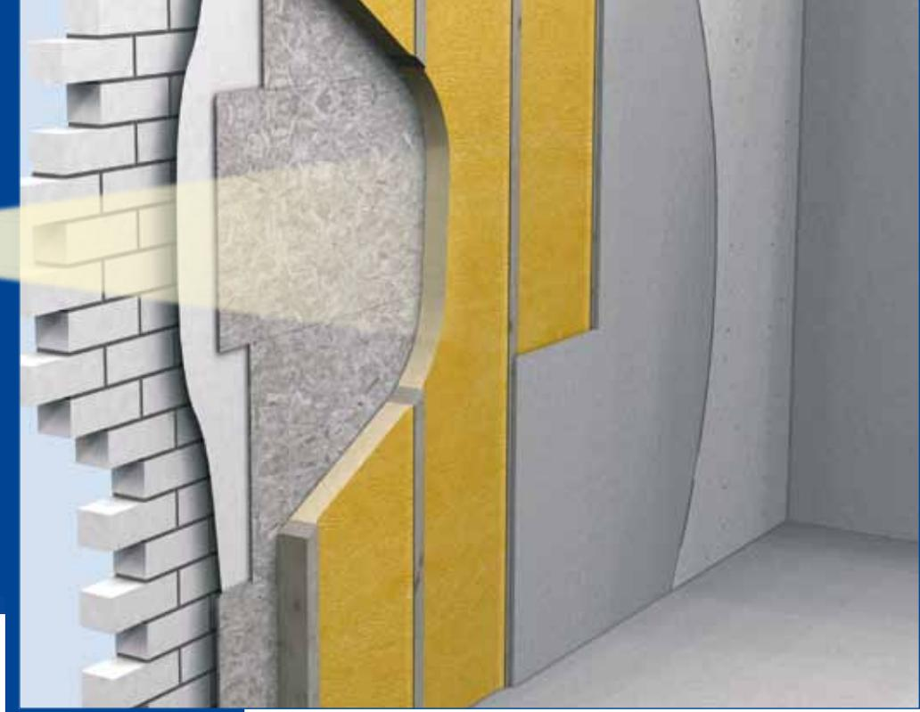
Timber frame construction is typical in Great Britain, USA and Canada. As the name suggests, this method of construction relies on a timber frame as a basic means of structural support. The outer leaf is typically stone, brick, render or timber, to suit the local district or planning requirements.
