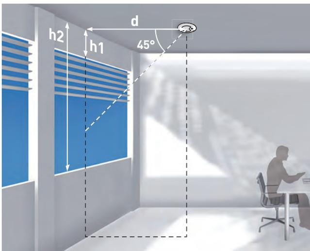
For optimum light level measurement, the sensor must be positioned between a minimum distance (to be determined) and 4 metres maximum from the source of natural light (large or small window, etc.). The ideal distance is calculated using the formula  $d = (h1 + h2) / 2$ .
