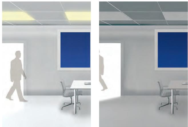
Sensors will switch on lighting automatically when a person enters the room, and switch lighting off automatically when no movement is detected.
